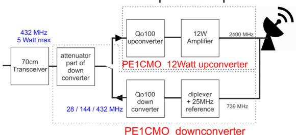
Simplex setup: the RX/TX switch and attenuator is implement in the downconverter
