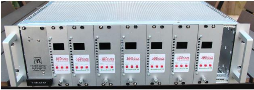
(photo: rack with 230V power supply. 1x talkback and 6x thru diversity broadband receiver.)
