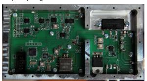
30 MHz Working range Number of channels 16 Deviation 40 or 50 kHz Audio bandwidth 15 kHz Audio input on demand 5mV up to 10 dBU > 70 dB Signal to noise Programming RS232 9600 baud. RF out SMA connection.
